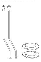
Two floor-stand posts, with "knurled" nuts, cone-shaped fittings, and 19mm-long hex head bolts installed.
